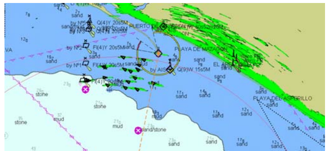
Figure 9. Radar Overlay correctly aligned with displayed chart
