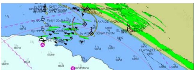
Figure 7. Radar Overlay not aligned with displayed chart
