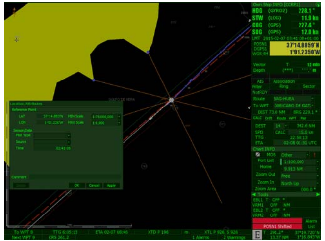
Figure 16. Observed position fixed on JRC ECDIS with use of LOP function
