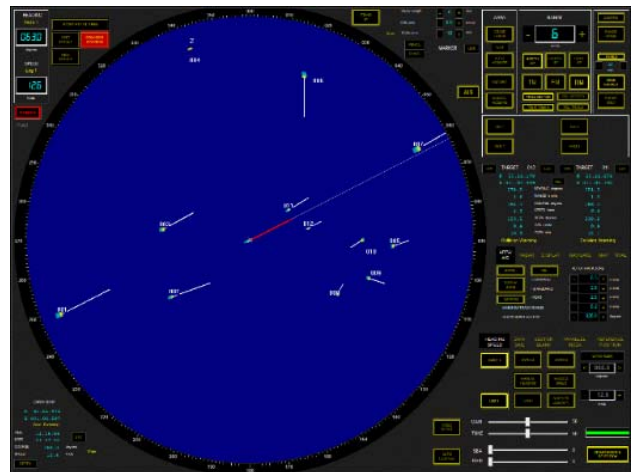
Figure 3. Own ship is in an overtaking situation in open waters where it is required to give-way. The situation is of high complexity as there are restrictions to own ship's avoidance manoeuvrability (both port and starboard).
