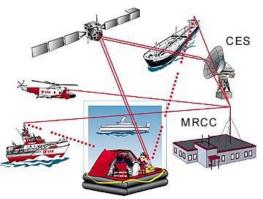
Fig.2. Inmarsat system communication.
