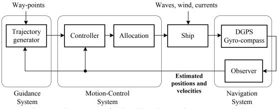
Figure 1. Basic components of modern ship motion control system (Fossen, 2002).
