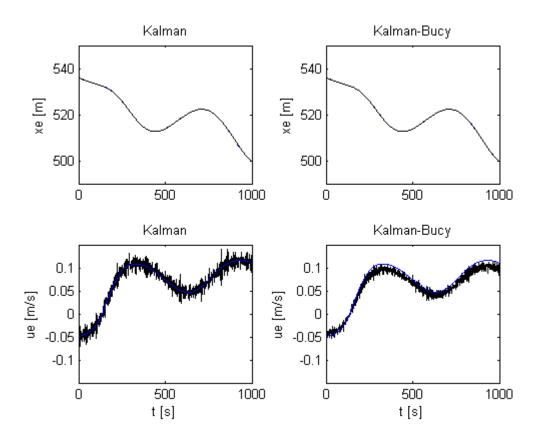
Figure 4. Simulation study: actual position with estimate and actual (black) and estimated (blue) velocity *u* in surge. Left-hand column – discrete Kalman filter, right-hand column – continuous Kalman-Bucy filter.
