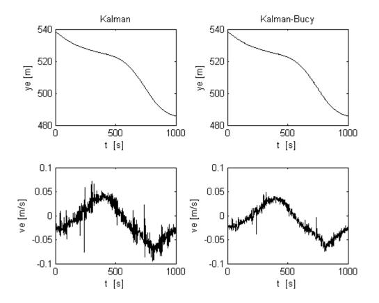
Figure 8. Experimental data: measured position with estimate and estimated velocity *v* in sway. Left-hand column – discrete Kalman filter, right-hand column – continuous Kalman-Bucy filter.
