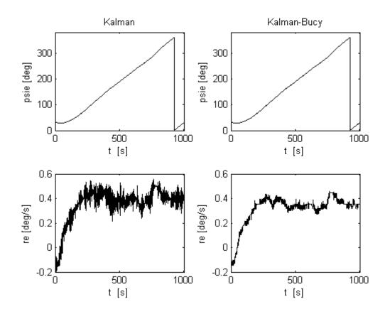
Figure 9. Experimental data: measured heading angle  $\psi$  with estimate and estimated angular rate *r* in yaw. Left-hand column – discrete Kalman filter, right-hand column – continuous Kalman-Bucy filter.
