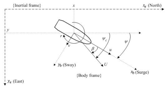
Figure 3. Variables used for describing ship motion.
