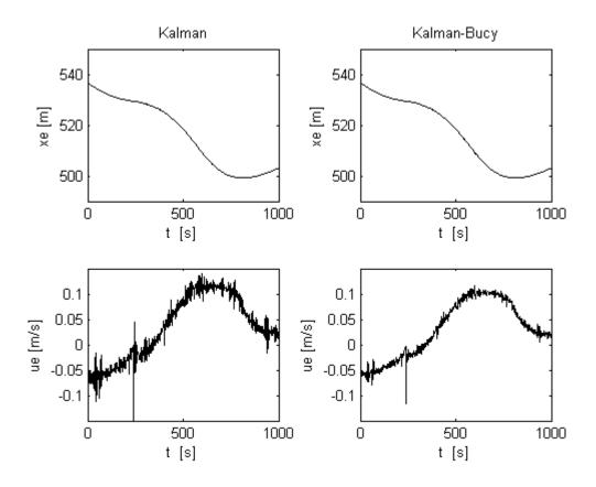
Figure 7. Experimental data: measured position with estimate and estimated velocity u in surge. Left-hand column – discrete Kalman filter, right-hand column – continuous Kalman-Bucy filter.
