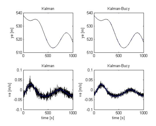
Figure 5. Simulation study: actual position with estimate and actual (black) and estimated (blue) velocity v in sway. Left-hand column – discrete Kalman filter, right-hand column – continuous Kalman-Bucy filter.
