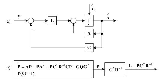
Figure 2. Block diagram of the continuous Kalman filter.
