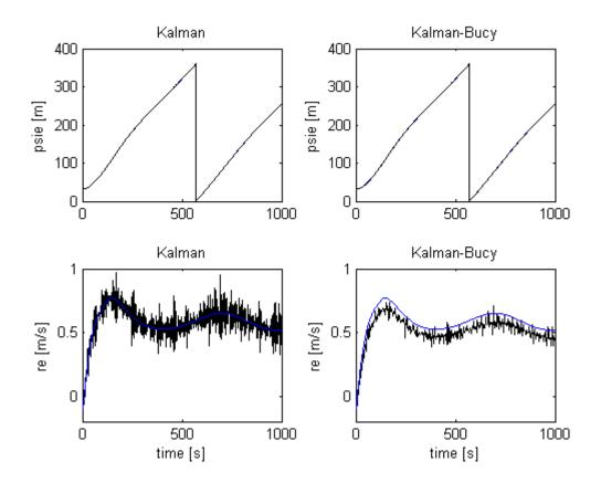
Figure 6. Simulation study: actual heading angle  $\psi$  with estimate and actual (black) and estimated (blue) angular rate *r* in yaw. Left-hand column – discrete Kalman filter, right-hand column – continuous Kalman-Bucy filter.
