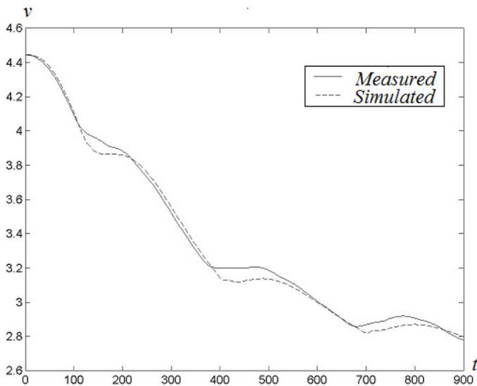
Figure 8. Speed comparison in 20/20 Zig-zag test
