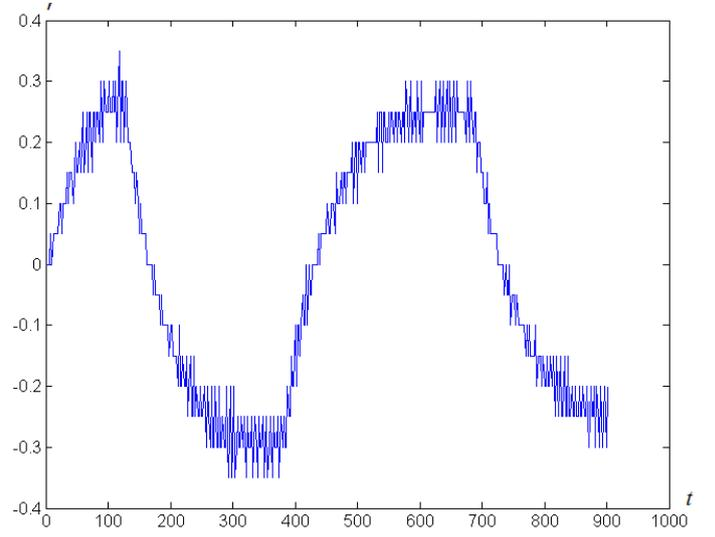
Figure 2. Rate of turn calculated from raw data.
