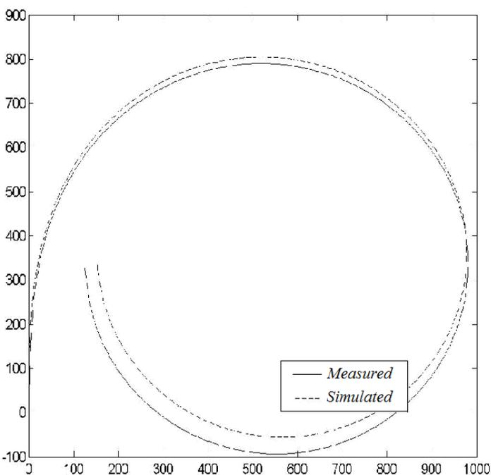
Figure 9. Turning circle comparison
