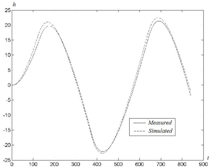
Figure 7. Heading comparison in 20/20 Zig-zag test
