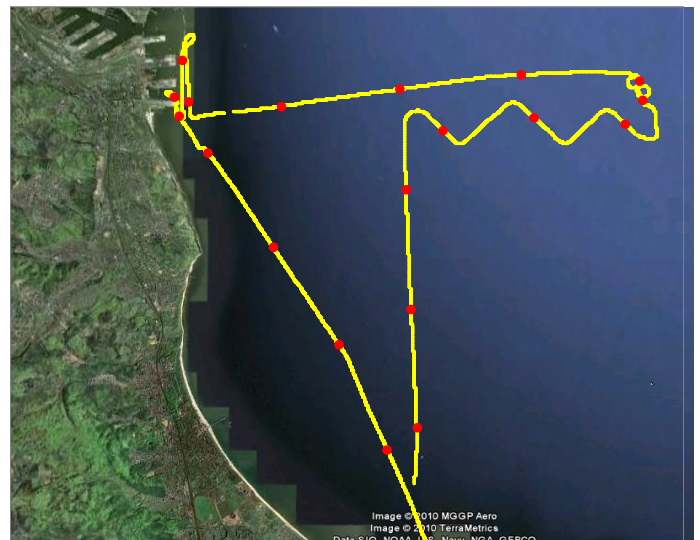
Figure 3. Complete track of the ship “Zodiak” during the measurements showing its positions received from onboard DGPS MX 420 receiver.
