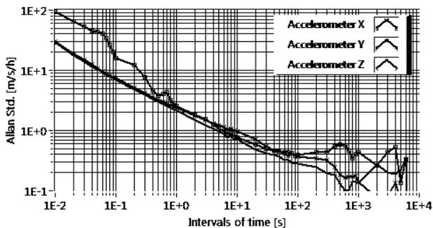
Figure 3. Allan standard deviation of the accelerometers measured in the LITEF  $\mu$ IMU.
