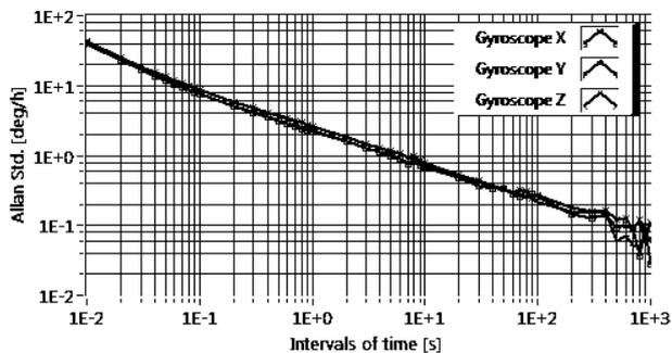
Figure 2. Allan standard deviation of the gyroscopes measured in the LN-200 IMU.
