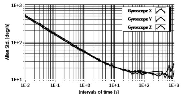
Figure 6. Allan standard deviation of the gyroscopes measured in the Xsens MTi-G710.
