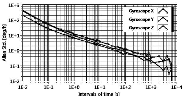
Figure 4. Allan standard deviation of the gyroscopes measured in the LITEF  $\mu$ IMU.
