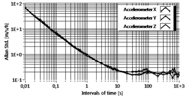
Figure 1. Allan standard deviation of the accelerometers measured in the LN-200 IMU.
