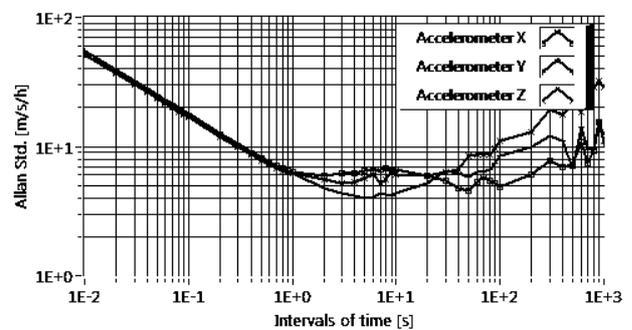
Figure 5. Allan standard deviation of the accelerometers measured in the Xsens MTi-G710.
