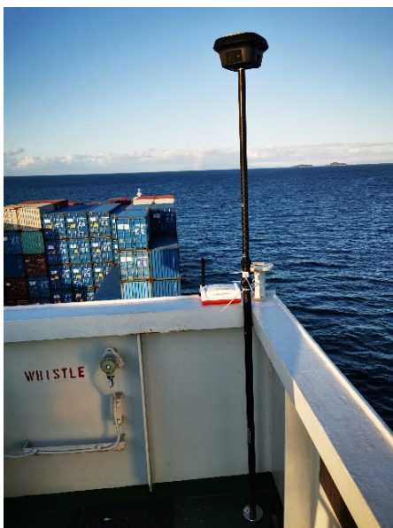
Figure 3. DGPS unit and PPU (Portable Pilot Unit) receiver on bridge wing
