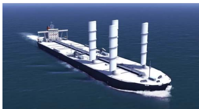
Figure 1. Automatically set rigid sails support the ship's propulsion [3]
