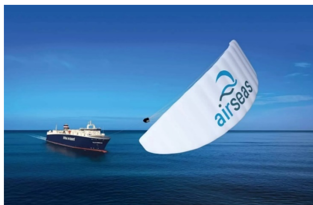
Figure 2. A kite-sail supports the main propulsion of the ship [4]
