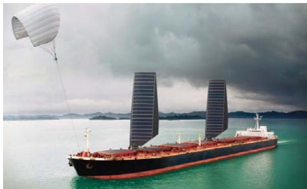
Figure 4. The use of photovoltaic panels and a kite-sail to reduce the ship's energy demand [6]
