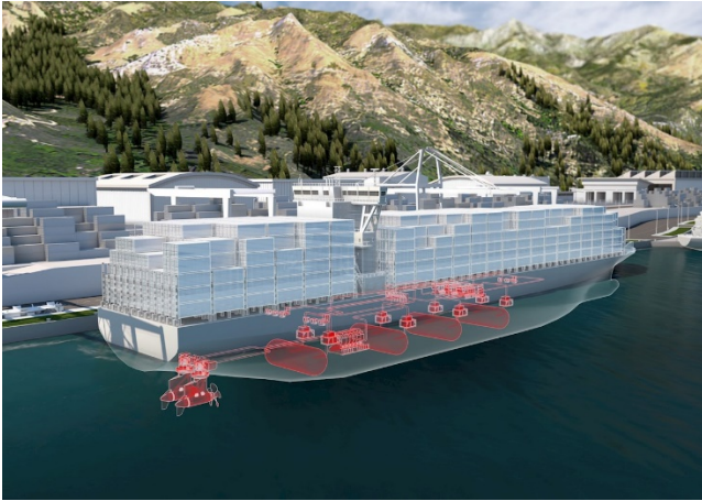
Figure 6. Concept illustration of a large vessel powered by fuel cells [8]
