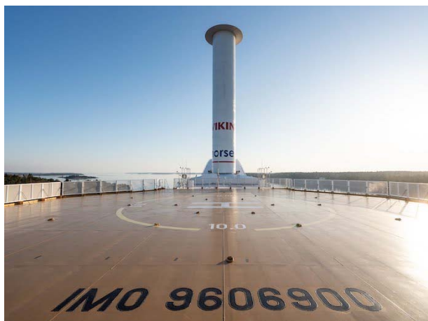
Figure 3. Norsepower designed and developed Rotor Sail. Flettner rotor produces an additional thrust to support the propulsion system of the ship [5]
