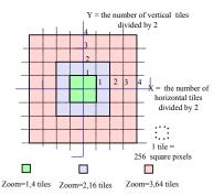
Fig. 2. Splitting grid at different zoom level
