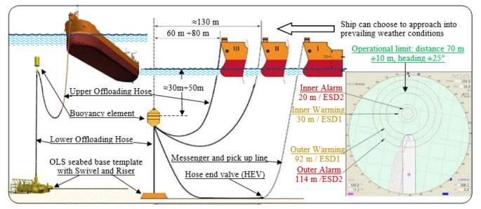
Figure 4. The Offshore Loading System OLS sometimes denoted also as UK-OLS, which stands for Ugland-Kongsberg OLS system with clearly marked operational zone preferred loading distance  $70m \pm 10$  m, inner and outer warmings and alarm limits for ESD1 and ESD2 procedure setup for DP shuttle tankers with Bow Loading System BLS based on OLS Operational Procedure [1], [6].
