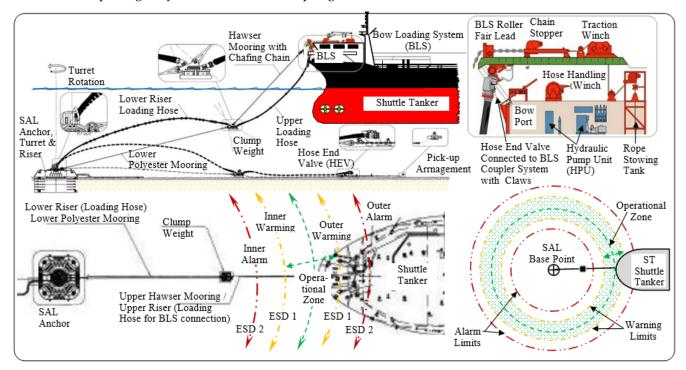
Figure 2. The Single Anchor Loading (SAL) system in Clump Weight configuration with safe operational zone, inner and outer warmings and alarm limits setup for ESD1 (Stop loading procedure) and ESD2 (Stop loading + disconnection procedure) for DP shuttle tankers with Bow Loading System (BLS) based on SAL Clump Weight Operational Procedure [1], [6].
